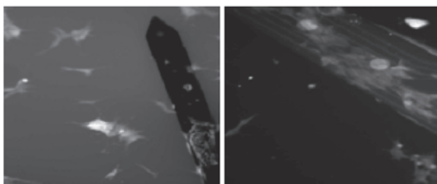
Fig. 8. Two neural probes cultured with human neuroblastoma cells: (left) uncoated; (right) PEDOT-MeOH/CDPGYIGSR coated.
